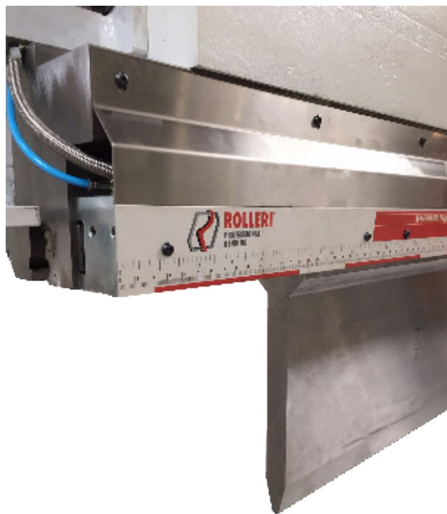
SPECIAL HYBRID SYSTEM (Pneumatic and Hydraulic) 500 Tons/meter
